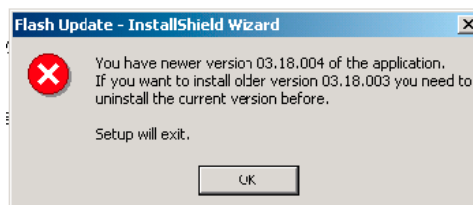
Figure 23 Flash installation interrupted
